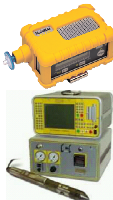
Fig. 2 – VOC sensor and Membrane interface Probe.
