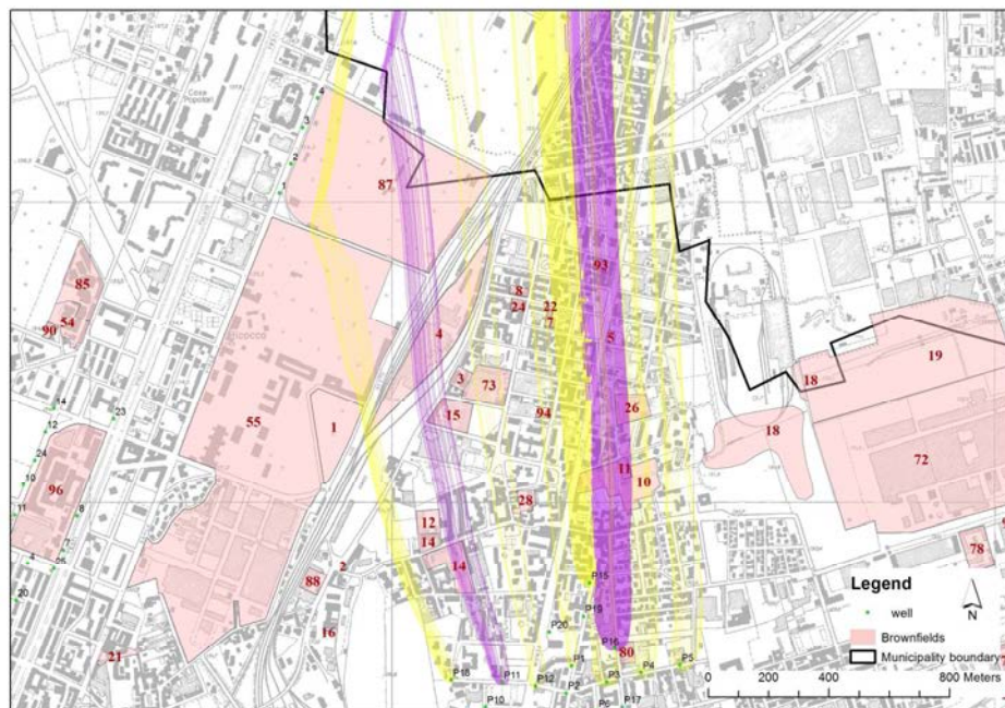
Fig. 1 – Particle backtracking (yellow and violet lines). Violet lines show the particle backtracking for P11 and P16, in which the highest mass flow rates, respectively of Freon 141b and CrVI, were detected. The pink areas are the known brownfields located upstream the pilot area.
