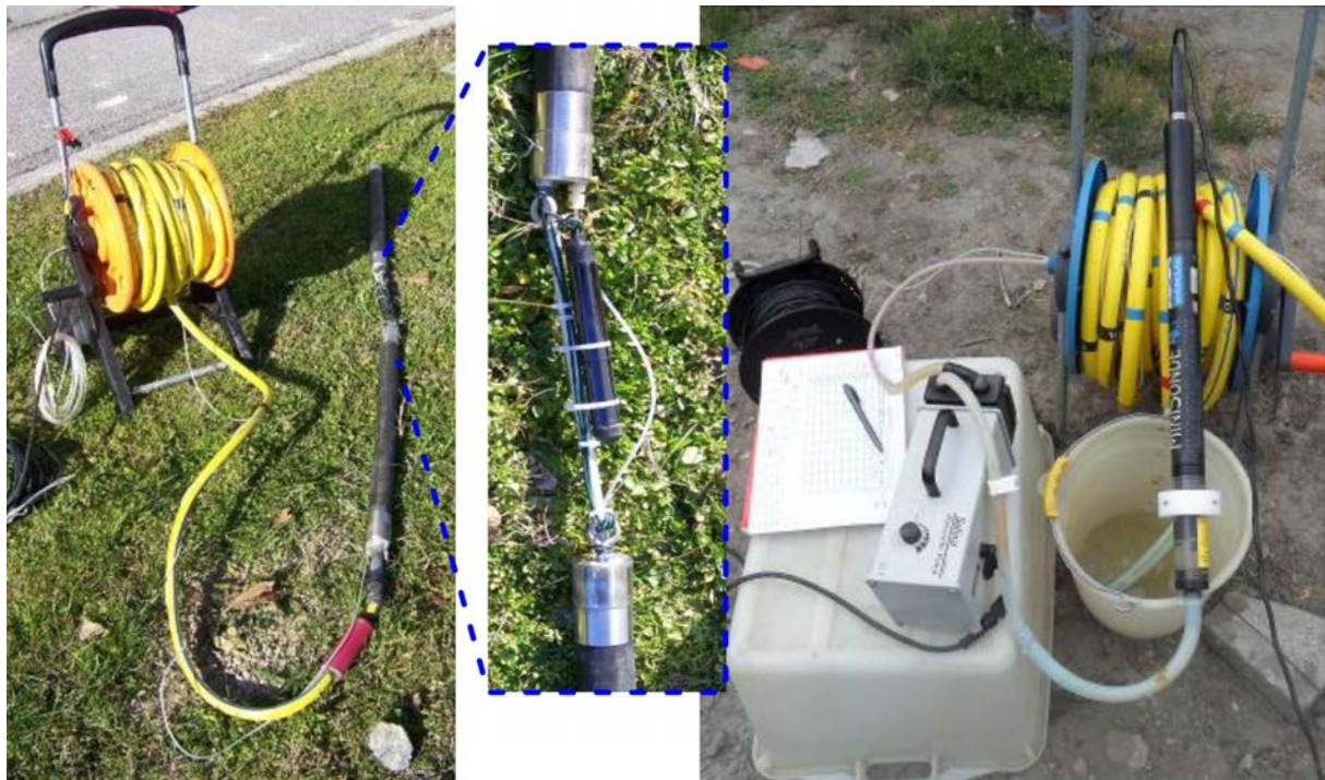
Fig. 1 – on the left the modified straddle packers with Levellogger positioned within the sampling window; in the center a zoom of the sampling window and on the right the Hydrolab flow cell for the monitoring of hydrochemical parameters.
