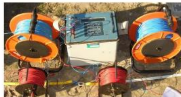
Fig. 2. Syscal PRO Equipment (IRIS Instruments - France) for Vertical Electrical Soundings (VES)
