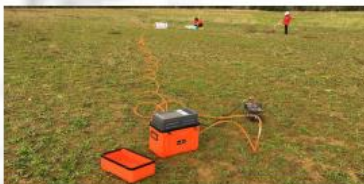
Fig. 7. Stratagem equipment (GEOMETRICS - U.S.A.) for magnetotelluric measurements
