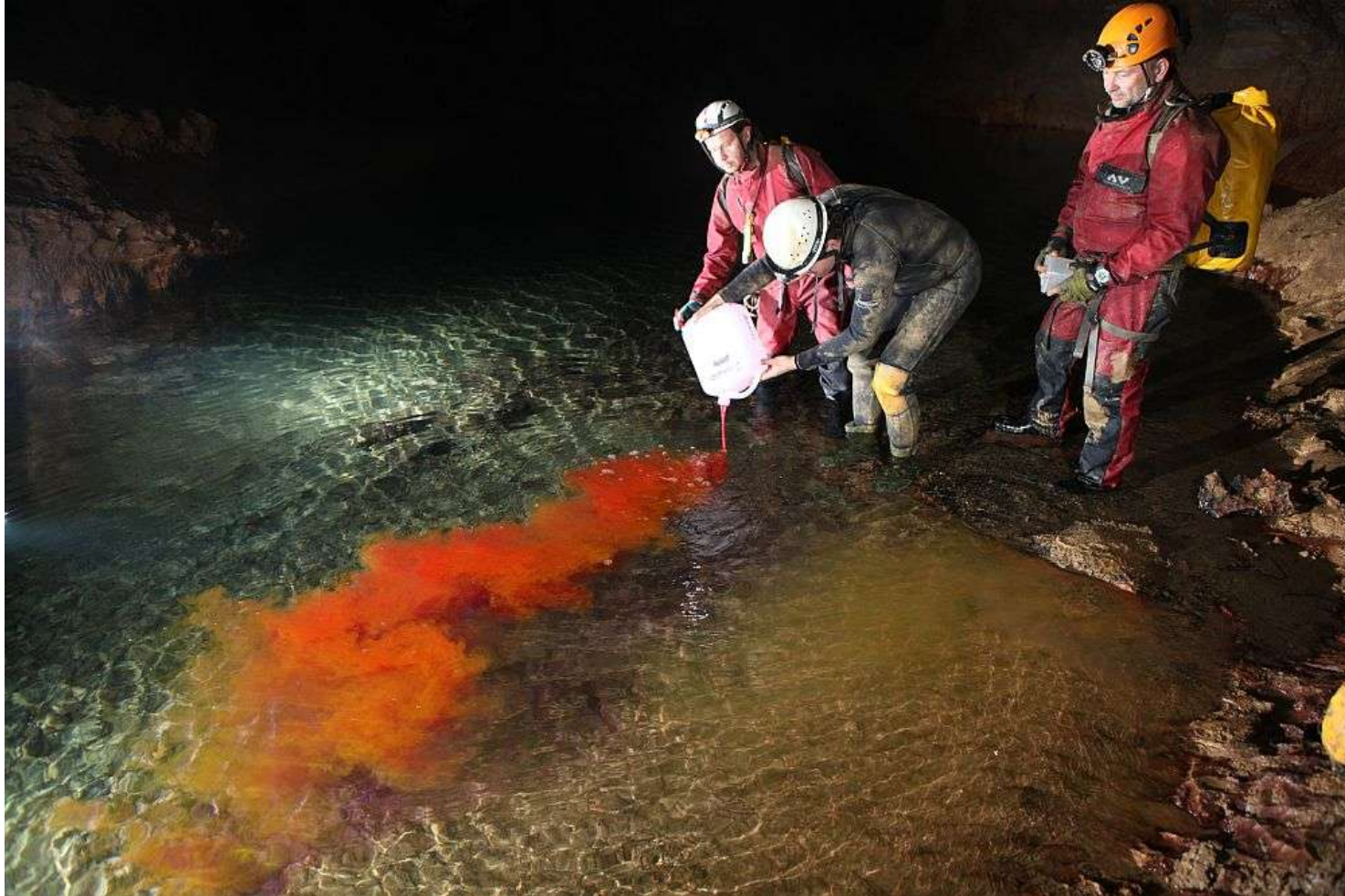
Injection of a fluorescent dye (Amidorhodamine) into Blauhöhle cave stream, Germany
