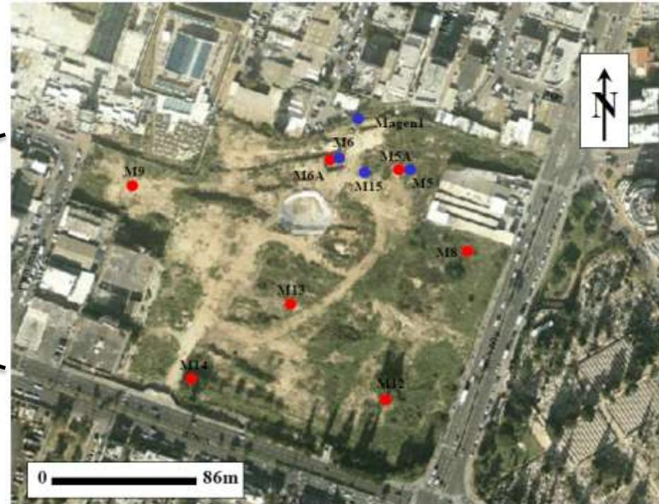
Existing monitoring wells at the Magen study area sampled in the course of this study; (●) wells that penetrate into the UZ; (●) wells that penetrate into both the saturated and unsaturated zones.
