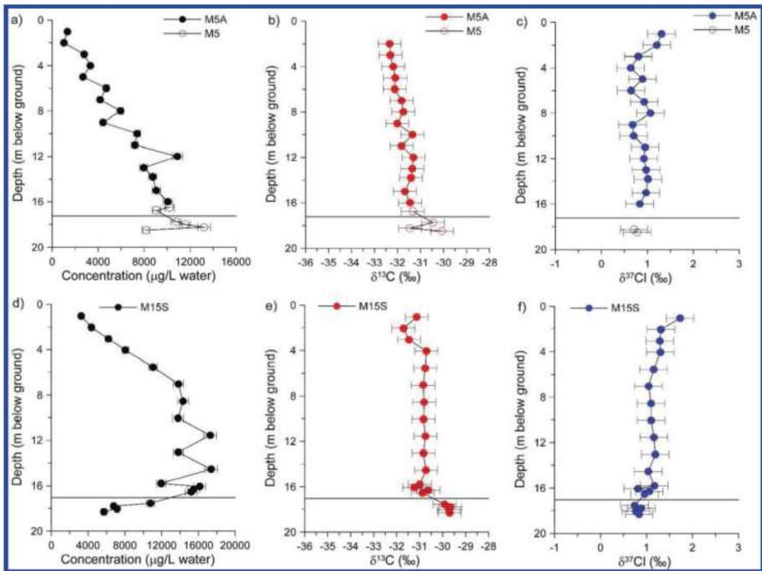
Concentration, stable carbon isotope ratio, and stable chlorine isotope ratio of TCE in monitoring wells M5A and M5 (a-c), and M15S (d-f). The concentrations in the unsaturated zone correspond to equivalent aqueous phase concentrations. The horizontal line indicates the location of the water table
